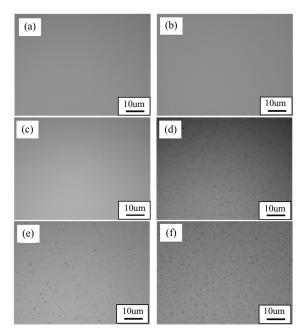
**Fig.8.** OM images of the thin films, sputtered by the 5N high purity aluminum target with sputtering rate 29.75Å/sec, were heat treated at various temperature for 1 minute. (a) without heat-treatment, (b)  $150^{\circ}$ C, (c)  $200^{\circ}$ C, (d)  $250^{\circ}$ C, (e)  $300^{\circ}$ C, (f)  $400^{\circ}$ C.
