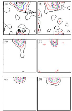
**Fig.4.** The ODFs ( $\Phi_2$ =45°) of 5N high purity aluminum hot rolled at 250°C, and then heat-treated at various temperature for 1 hour. (a) as-rolled,(b) 100°C, (c) 200°C, (d) 300°C, (e) 400°C, (f) 500°C.
