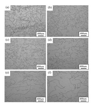
**Fig.1.** OM images of 5N high purity aluminum hotrolled at various temperature. (a) 150°C, (b) 200°C, (c) 250°C, (d) 300°C, (e) 325°C, (f) 350°C.
