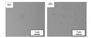
**Fig.10.** OM images of the thin films, sputtered by the 5N high purity aluminum target with sputtering rate 16.93Å/sec, were heat treated at various temperature for 1 minute.(a) 100°C, (b) 150°C.
