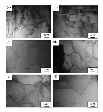
**Fig.5.** TEM images of 5N high purity aluminum hot-rolled at 250°C, and then heat-treated at various temperature for 1 hour. (a) as-rolled,(b) 100°C, (c) 200°C, (d) 300°C, (e) 400°C, (f) 500°C.
