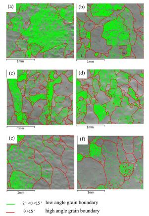
**Fig.3.** EBSD images of 5N high purity aluminum hot-rolled at 250°C, and then heat-treated at various temperature for 1 hour. (a) as-rolled, (b) 100°C, (c) 200°C, (d) 300°C, (e) 400°C, (f) 500°C.
