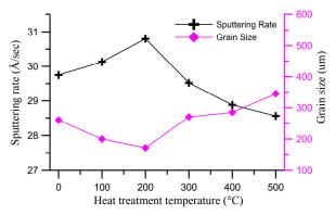
**Fig.7.** Correlation diagram between sputtering rate, heat-treatment temperature and grain size of 5N high purity aluminum hot-rolled at 250°C.
