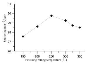
**Fig.6.** Correlation diagram between sputtering rate and finishing rolling temperature of 5N high purity aluminum.
