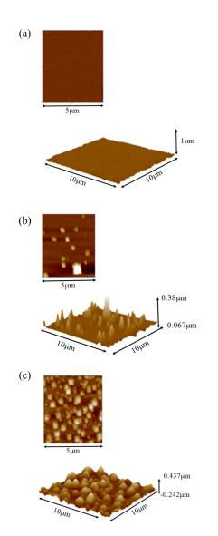
**Fig.12.** The AFM observations of aluminum thin film which were heat-treated at various temperature for 1 minute. (a) without heat-treatment, (b) 300°C, (c) 400°C.
